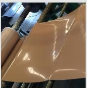
Pure Gum Rubber is used for a wide range of applications including seals and gaskets, vessel lining, diaphragm seals, vacuum blankets, pads and strips.
